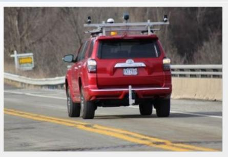
The technology used was the Deck Top Scanning System (DTSS) which is a mobile platform that can be loaded/mounted onto a vehicle. It consists of an infrared thermography (IR) camera, two line-scanning cameras, a GPS unit, and a speedometer unit that, combined, locate surface and sub-surface defects in bridge decks or roadways.
