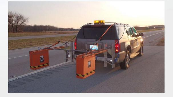
The technology used was a dual 2 GHz horn antenna system manufactured by GSSI, Inc. of Nashua, NH, The survey vehicle was equipped with an electronic distance-measuring instrument (DMI) mounted to the rear wheel of the survey van, providing continuous distance data as the GPR data was collected. The data collection and recording was controlled by the SIR-30 GPR system operated from within the survey vehicle.
